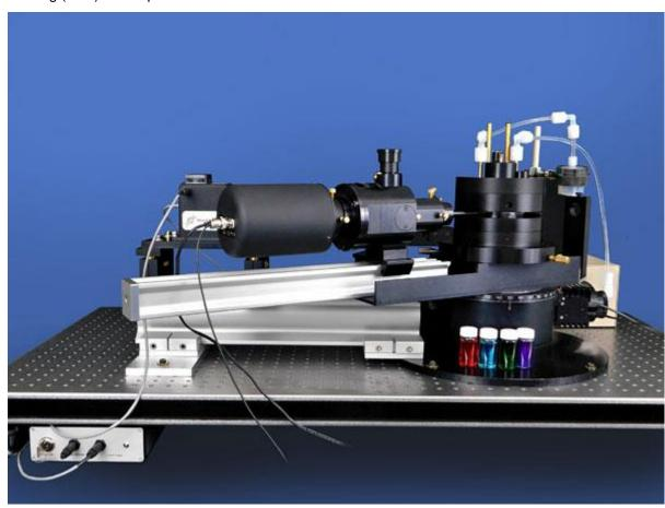
Traditionally, selection of the most appropriate wavelength for SLS or DLS applications has necessitated replacement of one laser with a different one, a time-consuming operation requiring precision re-alignment work. Alternatively, users could elect to employ a single, very costly multi-wavelength Ar-Ion laser in their light scattering goniometer system.
